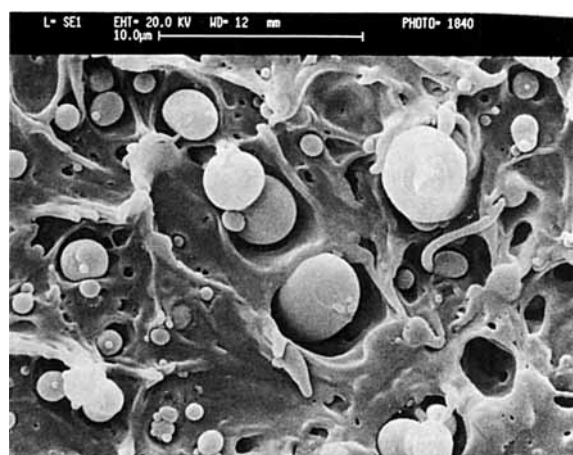
Figure 19 Scanning electron micrographs of extrudates of PP/SEBS/PC ternary blend at a fixed composition 90/10/10 and shear rate ( s^{-1} ): 2 \times 10^3 .
